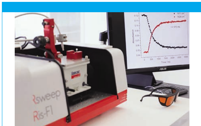
Figure 1: Set-up: IRis-F1 dual-comb spectrometer with ATR Golden Gate for \mu\text{s/ms} reaction monitoring; 40 Hz for curing was applied.
